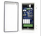
PCR43304RE 4-Channel Receiver enclosed in an IP66 case
