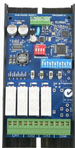
PCR43304R 4-Channel Receiver with Relay Outputs
