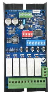
PCR43305R 5-Channel Receiver with Relay Outputs
