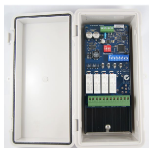
PCR43304RE 4-Channel Receiver enclosed in an IP66 case
